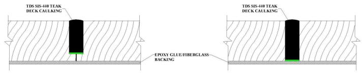
Use of polyurethane bond breaker tape in seams of 6mm and deeper. It aids to achieve 2-sided adhesion. The bottom of seam must be flat and square. The caulk seam should be able to move at the base of the seam, as the deck flexes and works.
